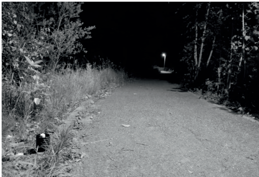
Figure 2 A LED trap (lower left) in an illuminated area beneath a street lamp. Another trap (not visible) is placed in the dark area between this and the next street lamp in the distance.
